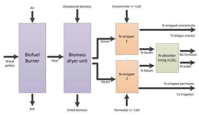
Figure 3. Simplified overview of the biomass dryer unit and the nitrogen stripper units of the New Substrate Concept.
