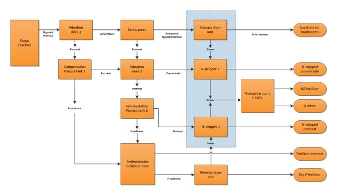
Figure 2. Overview of the different components in the complete New Substrate Technology Concept. Note that in most cases only one biomass dryer unit will be included since one dryer unit normally will have sufficient capacity to treat both the dewatered digested biomass and the P-sediment. The present verification focusses on the key components highlighted in the blue box: 1) The biomass dryer unit (drum dryer) including a biofuel burner unit. 2) The two N-stripper units.
