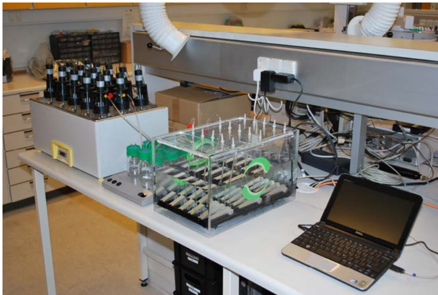
Laboratory setup for measurement of biogas and methane production of different substrates.
