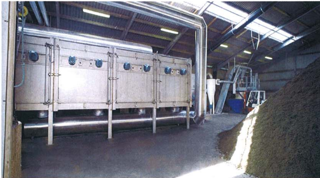
Figure 3. SHSD - Super Heated Steam Drier.
