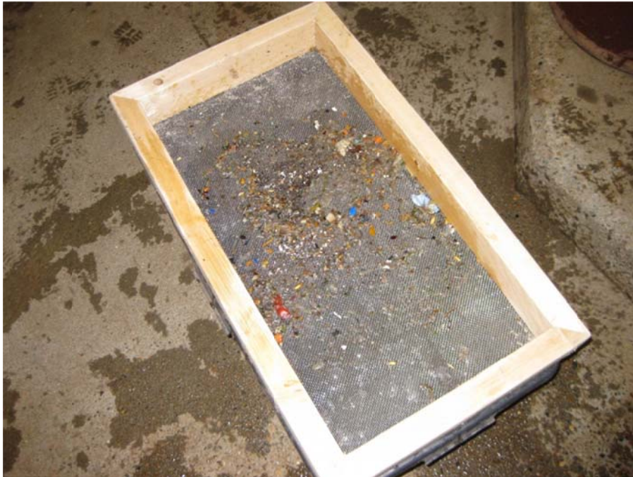
Figure 9 Collection of 2 - 10 mm reject from washing
