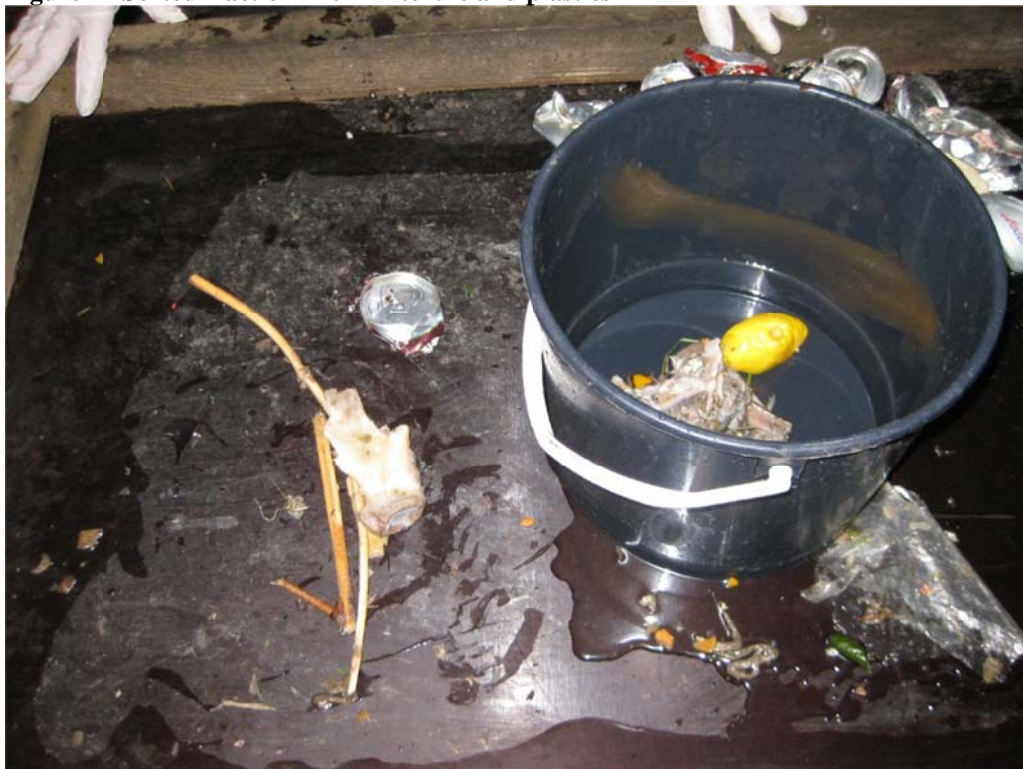
Figure 15 Sorted fraction >40 mm metal, organic residue and non biogas degradable woodsticks and bones
