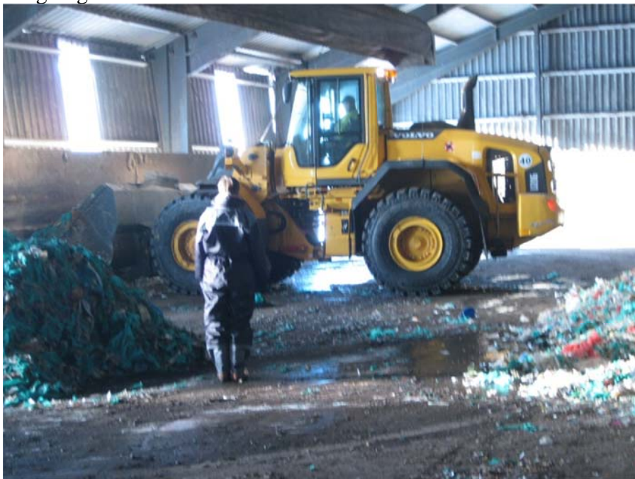
Figure 6 Mixing of 3 batches to one sample representing a test run and weighing with wheel loader
