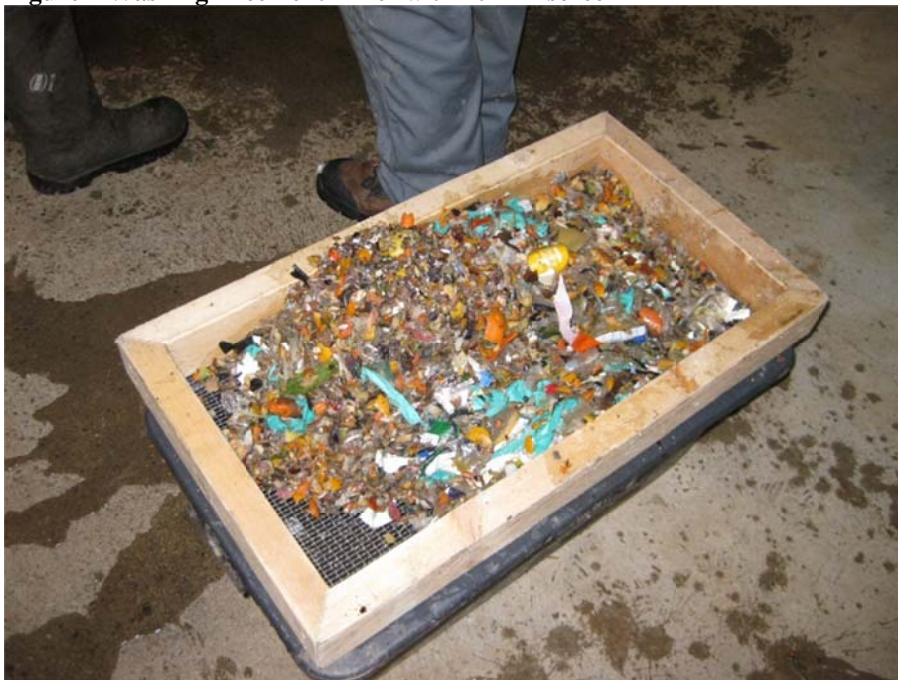
Figure 8 Collection of 10 - 40 mm reject from washing
