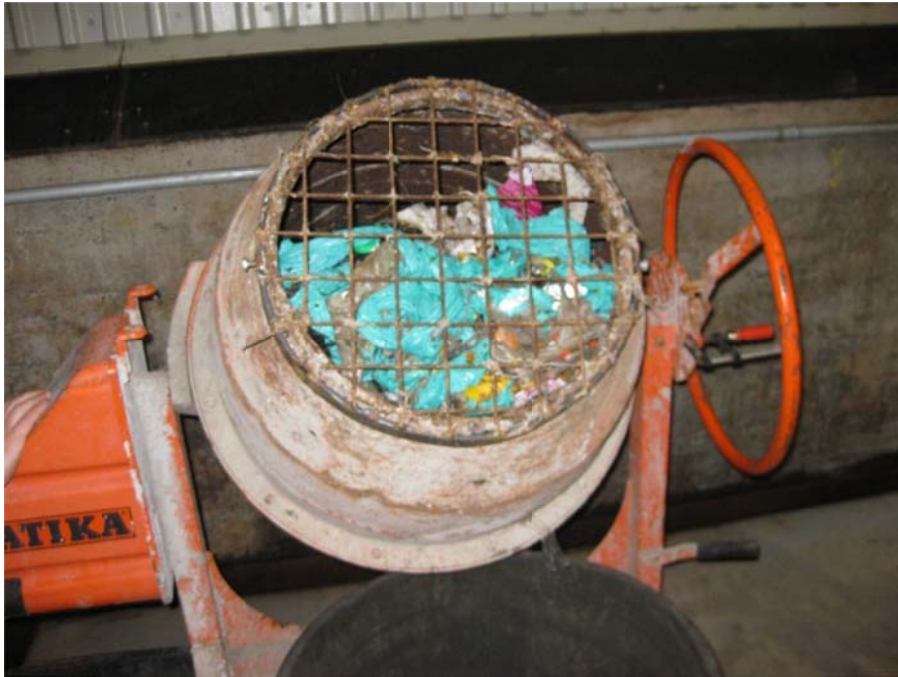
Figure 7 Washing in cement mixer with 40 mm screen
