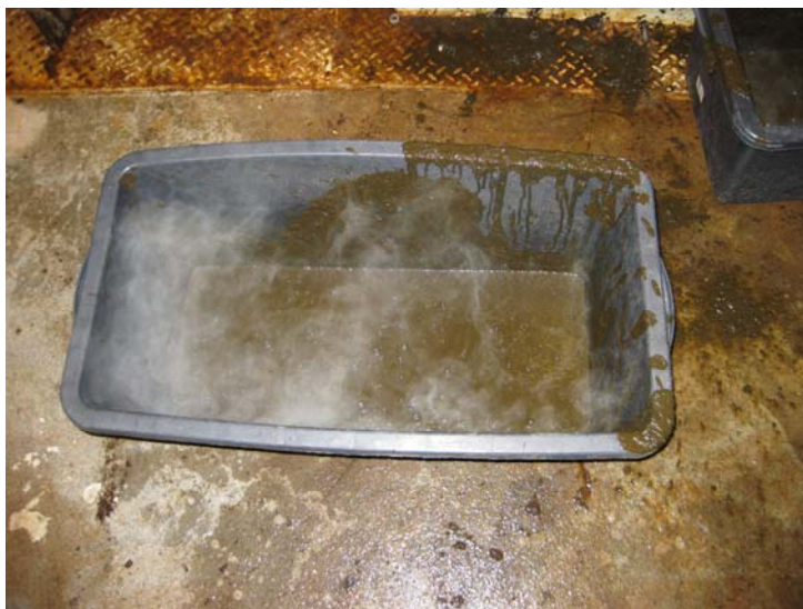
Fig 3. Sampling of pressure-cooked biomass into a 60 l container
