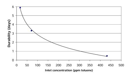
The curve shows that the durability increases with lower concentration.
