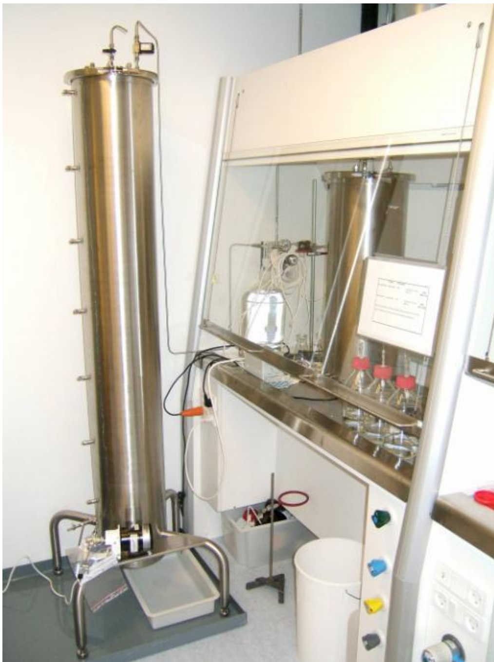
Figure 5 Standpipe. The air wash bottle is in the fume cupboard.
