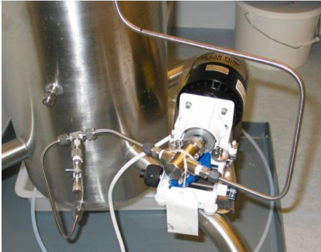
Figure 6 Detail of standpipe: recirculation pump and spiking port.
