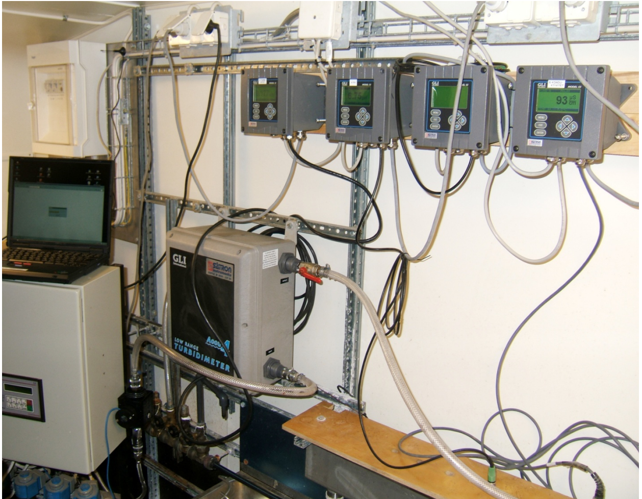
Figure 2-5 View into the trailer with analytical equipment. In the lower right corner is the flow-through channel with the sensors.
