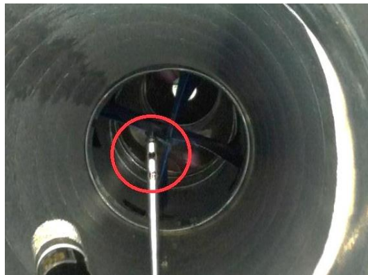
Figure 2 - Visually inspect the hotwire anemometer
