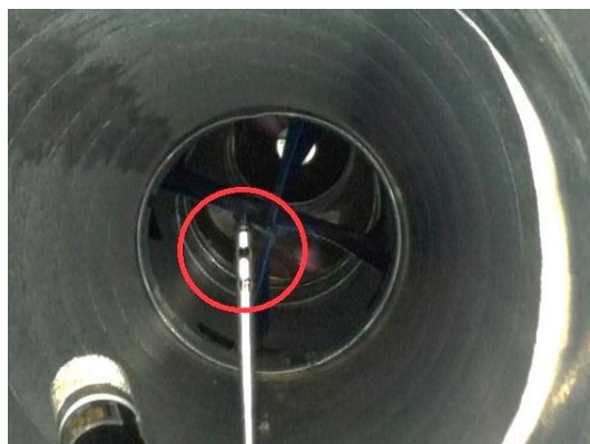
Figure 2 - Visually inspect the hotwire anemometer
